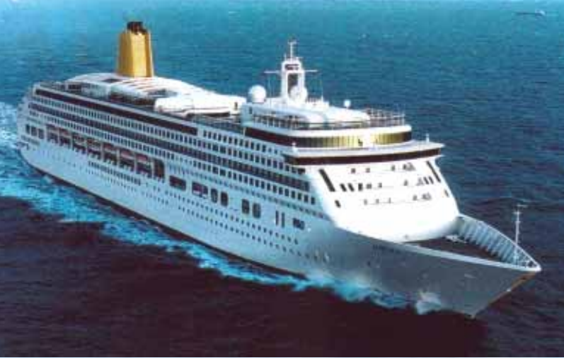
Cruise Liner driven by 20,000 kW Variable Speed Synchronous Motors
