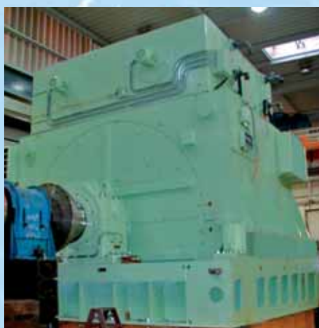
Variable Speed Synchronous Motor for Cruise Liner
